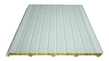
Roduction Plant: Balıkesir Favourable Width: 1000 mm Minimum Length: 3 meters Maximum Length: Depends on Transport Conditions Mineral Wool Density: 100 (±10) kg/m<sup>3</sup> Mineral Wool Thickness: 50-60-70-80-100-120-130-150 mm Heat Insulation Coefficient: 0,033 W/mK Inflammability Class (EN 13501-1): A1 Water Absorption: 2% by Volume Heat Resistance: 600 °C Sound Insulation Rw [dB]: 30 Water Vapor Diffusion (EN 12086): 1
