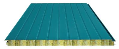
Production Location: Balıkesir Modular Width: 1000 mm Minimum Length: 3 meters Maximum Length: Depends on transport conditions. Mineral Wool Density: 100 (±10) kg/m<sup>3</sup> Mineral Wool Thickness: 50-60-80-100-120-130-150 mm Thermal Conductivity Coefficient: 0.033 W/mK Inflammability Class (EN 13501-1): A1 Water Absorption: By Volume 2% Heat Resistance: 600 °C Sound Insulation Rw [dB]: 30 Water Vapour Diffusion (EN 12086): 1
