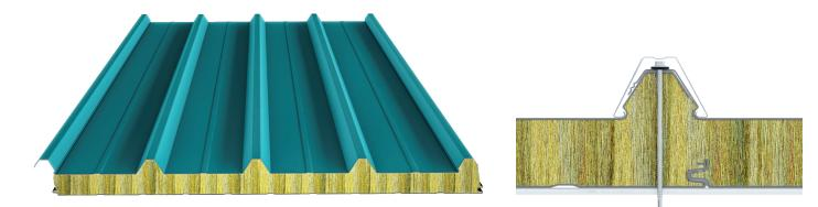
Production Plant: Balıkesir Favourable Width: 1000 mm Minimum Length: 3 meters Maximum Length: Depends on Transport Conditions Mineral Wool Density: 100 (±10) kg/m<sup>3</sup> Mineral Wool Thickness: 50-60-70-80-100-120-130-150 mm Heat Insulation Coefficient: 0.033 W/mK Inflammability Class (EN 13501-1): A1 Water Absorption: %2 by Volume Heat Resistance: 600 °C Sound Insulation Rw [dB] ≥: 30 Water Vapor Diffusion (EN 12086): 1
