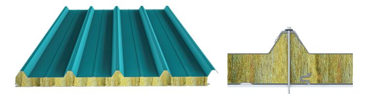
Production Plant: Balıkesir Favourable Width: 1000 mm Minimum Length: 3 meters Maximum Length: Depends on Transport Conditions Mineral Wool Density: 100 (±10) kg/m<sup>3</sup> Mineral Wool Thickness: 50-60-70-80-100-120-130-150 mm
