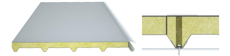
Production Plant: Balıkesir Favourable Width: 1000 mm Minimum Length: 3 meters Maximum Length: Depends on Transport Conditions Mineral Wool Density: 100 (±10) kg/m<sup>3</sup> Mineral Wool Thickness: 50-60-70-80-100-120-130-150 mm Heat Insulation Coefficient: 0.033 W/mK Inflammability Class (EN 13501-1): A1 Water Absorption: %2 by Volume Heat Resistance: 600 °C Sound Insulation Rw [dB] ≥: 30 Water Vapor Diffusion (EN 12086): 1
