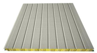
Production Location: Balıkesir Modular Width: 1000 mm Minimum Length: 3 meters Maximum Length: Depends on transport conditions. Mineral Wool Density: 100 (±10) kg/m<sup>3</sup> Mineral Wool Thickness: 50-60-80-100-120-130-150 mm Thermal Conductivity Coefficient: 0.033 W/mK Inflammability Class (EN 13501-1): A1 Water Absorption: By Volume 2% Heat Resistance: 600 °C Sound Insulation Rw [dB]: 30 Water Vapour Diffusion (EN 12086): 1
