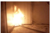
The contribution of the material in the expansion of the fire, even the resistance shown by the material against the fire which is also qualified as flammability capacity is called fire performance. A panel system formed of inflammable metal surface as well as polyurethane can be qualified as B,s2,d0 i.e. hard to burn according to EN 13501 norm, however evaluating the behavior of the fire to occur in the building over the fire performance of the wall coating material will be incomplete.
