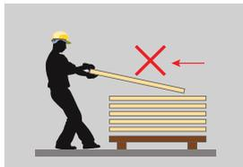
Do not drag panels in a pile, or on the roof purlins. Lift panels from both ends when moving or laying in place.
